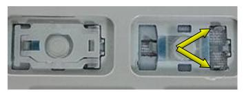
Next, press hinge into alternate mounts
