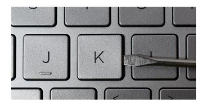
Removing broken hinge pieces is a much easier process, as you are able to see the connecting points and can use your tool to gently unclip or free the component from the mounting points on the keyboard. Again, the exact removal method will vary between models. Most hinges will attach via three or four mounting points located on the keyboard. Start by removing the hinge on the most accessible side and the remaining clips will come free.
