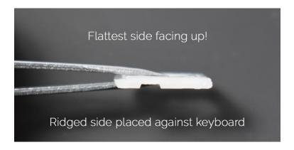
2. You'll also need to orient the hinge so it can be mounted correctly onto the keyboard. Most hinges can only be installed properly in one direction, so this is a fairly straightforward step. However, if you aren't sure of the correct orientation just double check your laptop model and hinge type on our website. Our images on each product page will show the correct orientation for every hinge available for that particular model.
