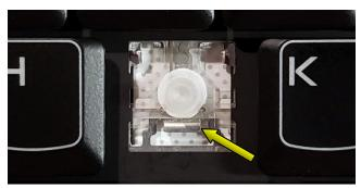
Install onto single lower mount first!
