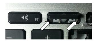
With the hinge now properly installed, you can place the optional rubber cup if needed. Apply a <u>small</u> amount of glue around the OUTER rim of the cup and seat it in the center of the hinge assembly. Sometimes the rubber cup will firmly sit in place by itself, but it is better to use adhesive.
