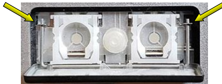
Corresponding slots/holes to accept the stabilizer bar
