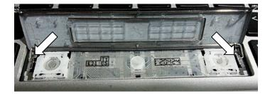
You can now attach the metal brackets on the key cap. To do so, simply place each bracket into their respective holes on the keyboard. If you cannot install these, the key cap can still be used without the stabilizer brackets. Once completed, you can rotate the key down into place. Keep the key cap centered over the installed hinges and press down. If the key cap clicks into place, you've finished the installation! Great job!
