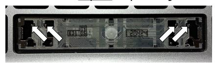
Hinges are pre-attached to each key for protection during shipping and must be removed to install. Take note of the orientation of the hinge mechanisms to help you with placement.
