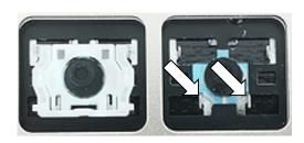
Hinges may be pre-attached to each key for protection during shipping and must be removed to install. Take note of the orientation of the hinge mechanism to help you with placement.
