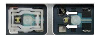
To install the hinge mechanism, begin by hooking one end over the protruding metal tabs located on the keyboard. A small flat screwdriver or blunt tweezers will assist you in this step.
