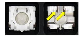
To install the hinge mechanism, begin by hooking one end over the protruding metal tabs located on the keyboard. A small flat screwdriver or blunt tweezers will assist you in this step.
