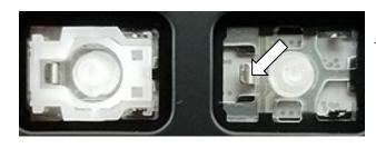
To install the hinge mechanism, begin by hooking one end over the protruding metal tab located on the keyboard. A small flat screwdriver or blunt tweezers will assist you in this step.
