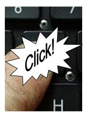
With the hinge now properly installed, you can place the optional rubber cup if needed. Apply a **small** amount of glue around the OUTER rim of the cup and seat it in the center of the hinge assembly. Sometimes the rubber cup will firmly sit in place by itself, but it is better to use adhesive. **Allow ample drying time before installing the key cap!** Then, simply place the correctly oriented key cap over the hinge mechanism and press down. If the key cap clicks into place, you're all done!
