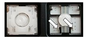
To install the hinge mechanism, begin by hooking one end over the protruding metal tabs located on the keyboard. A small flat screwdriver or blunt tweezers will assist you in this step. Keep the flattest side of the hinge facing up so it is able to properly receive the key cap.
