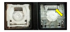
To install the hinge mechanism, begin by hooking one end over the large metal tab located on the keyboard. A small flat screwdriver or blunt tweezers will assist you in this step.
