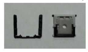
Hinges are pre-attached to each key for protection during shipping and must be removed to install. Take note of the orientation of the hinge mechanism to help you with placement.
