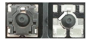
Hinges may be pre-attached to each key for protection during shipping and must be removed to install. Take note of the orientation of the hinge mechanism to help you with placement.
